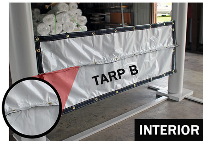
This is an inside view of Tarp B. It hangs from the cable. Take notice of the standing seam 1' down from the edge. This seam will be used to connect the flap from Tarp A to create the overlap.
